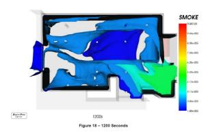
In this case, Fire Field (CFD) Modelling was carried out to show some of the typical worse case scenarios that could be experienced in enclosed Car Parks and the effectiveness of various mechanical ventilation systems in mitigating the effects of both fires and CO exhausts within the structure.
